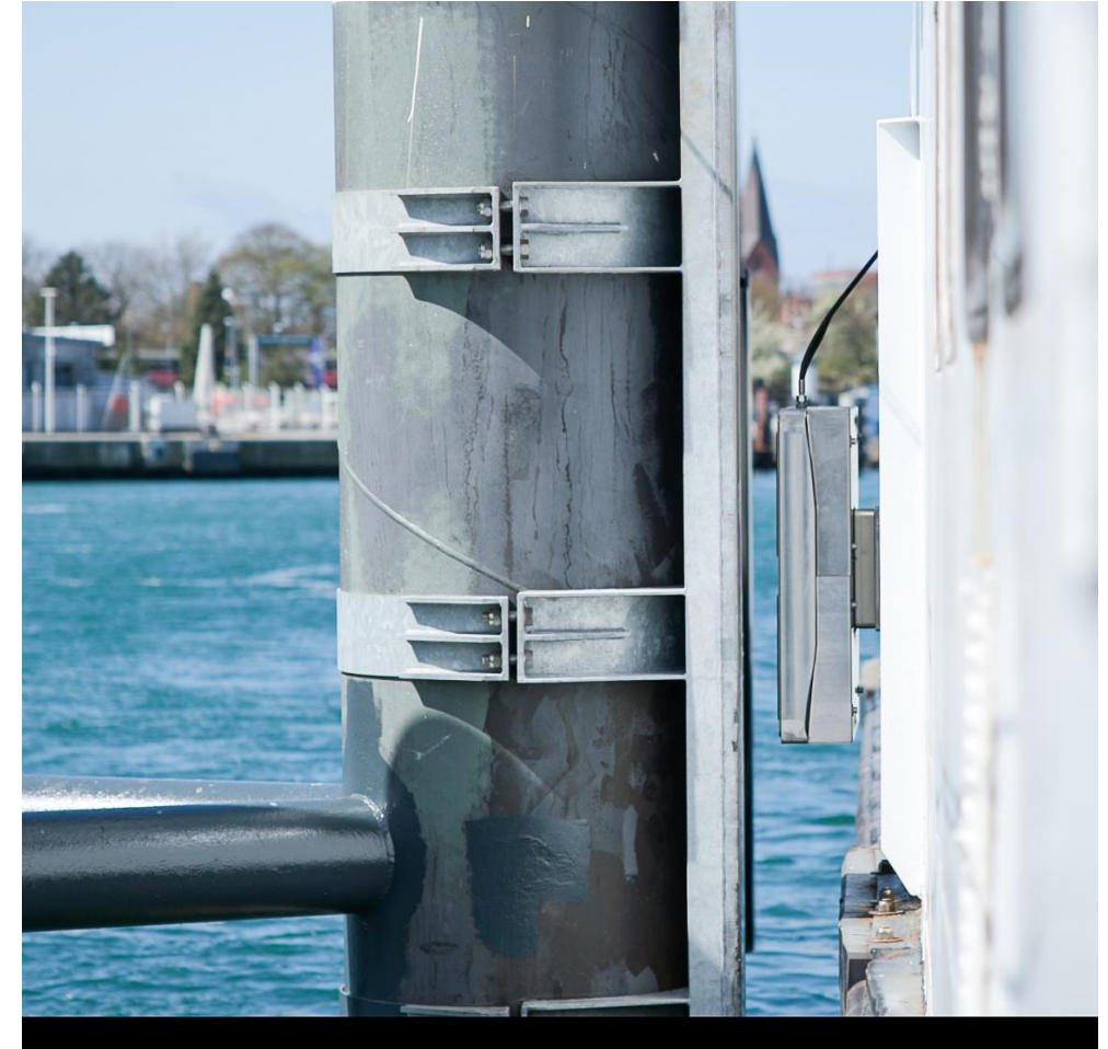
Magmoor on M/F Warnow and the counter plate at Hohe Düne, Germany.
